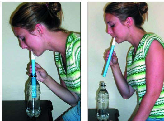
Figure 2. With the slide removed from the slide whistle, it can act as either a closed pipe with a variable length (when submerged in the water) or an open pipe (when out of the water).
