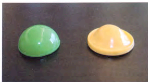
Figure 1. Two 1 inch plastic toy poppers. The one on the left is in its stable condition. The one on the right has been inverted. This causes an instability which will lead to it restoring itself to its stable condition. The restoration leads to a force being applied to the surface which leads to a 'pop' off the surface.
